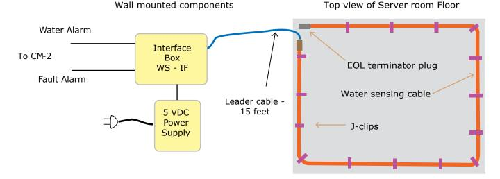
The WaterSnake's four components: the sensing cable, a leader cable, the interface box and a small power supply. The interface box and power supply are usually wall mounted. The sensing cable secures to the floor with plastic J-clips.
