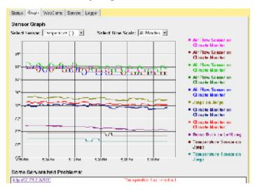
Superimpose sensor values from multiple devices. Quickly call out suspicious values. Devices that cannot be contacted are displayed at the bottom.
