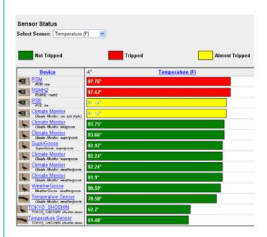
Graph views consolidate sensor data from multiple and mixed device types. Colors indicate which devices are in or close to an alarm state.
